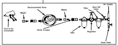
preferably incorporating a rust inhibitor. Reconnect tool to air supply and run tool slowly for a few seconds to allow air to circulate the oil. If tool is used frequently lubricate on daily basis and if tool starts to slow or lose power.
