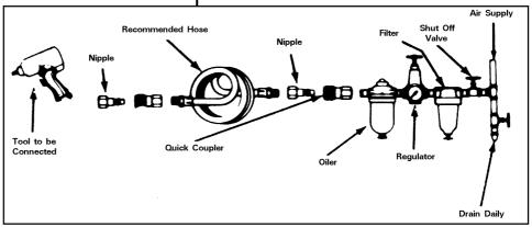
pressing the trigger on the tool. Disconnect the air line and pour into the intake bushing a teaspoonful (5ml) of a suitable pneumatic motor lubricating oil preferably incorporating a rust inhibitor. Reconnect tool to air supply and run tool slowly for a few seconds to allow air to circulate the oil. If tool is used frequently lubricate on daily basis and if tool starts to slow or lose power.
