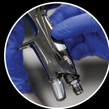
Use the Trigger Locking Clip and wash the spray gun
